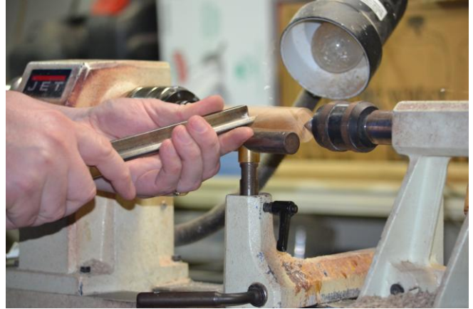
Using a spindle roughing gouge, round the blank and taper it towards the tail stock.
