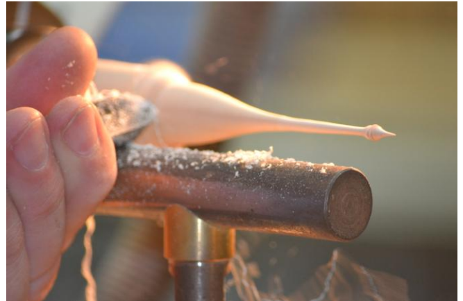
Now I am turning the onion bulb. Using the point of the gouge pointed down the curve of the bulb.
