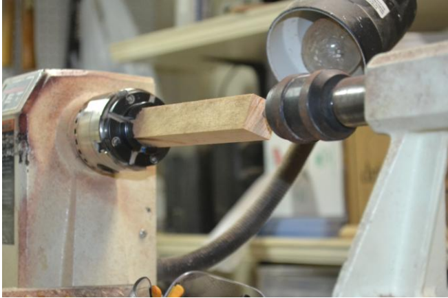
Mount a suitable blank in the jaws of a chuck (left square here) or you can turn a tennon between centers first.
