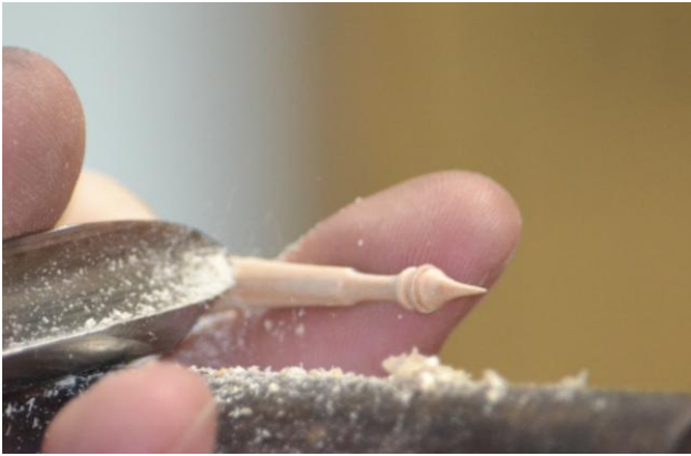
The terminal on this finial is a point with two very fine v-grooves cut below the point using a "Vortex" or point tool. Here I am working on the flat transition between the terminus and the onion bulb.
