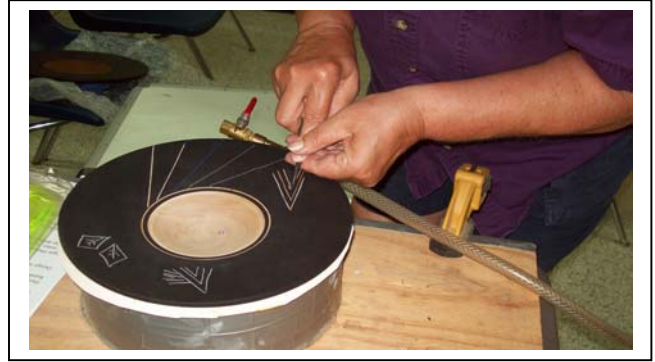
Hand carving lines in vacuum holder
