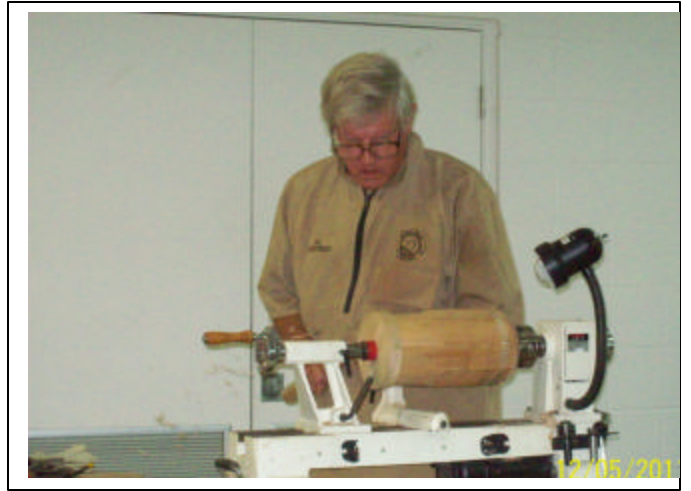
Turning the house staves
