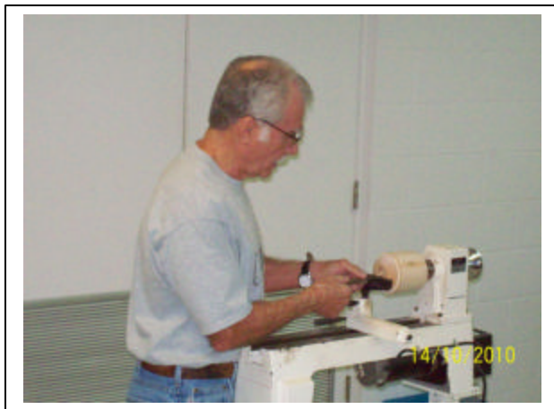
Turning out bottom in Jam chuck tape block (#2MT drive).
