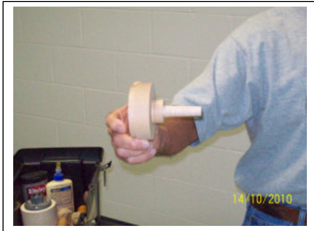
Disk on #2MT jam chuck (allows access on both sides)
